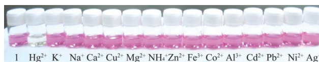
Fig. 2 Photograph of 10 \mu\text{M} 1 in the presence of different nitrate salts: (10.0 equiv) of Na + , K + , NH 4 + , Mg 2+ , Ca 2+ , Pb 2+ , Hg 2+ , Co 2+ , Cd 2+ , Zn 2+ , Ni 2+ , Cu 2+ , Cr 3+ , Fe 3+ and Ag + in H 2 O.
